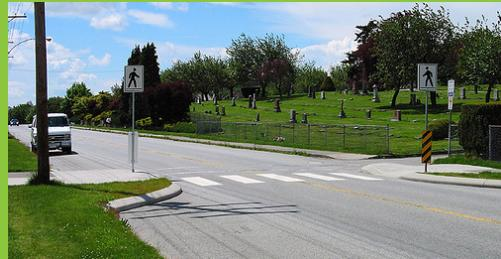
**Curb Extension (Curb Bump Outs):** A mid-block or intersection widening of the boulevard, which narrows the travel lane(s). Curb extensions may be used in conjunction with pedestrian crosswalks.
